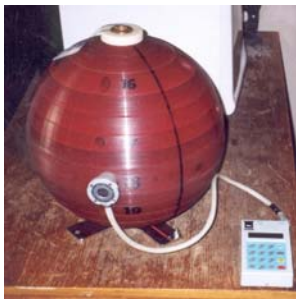
Fig.3 View of Liulin-5 inside the phantom during the tests of the instrument. In the center is seen the detector module mounted in the radial channel, while at the right side is the electronic block.
