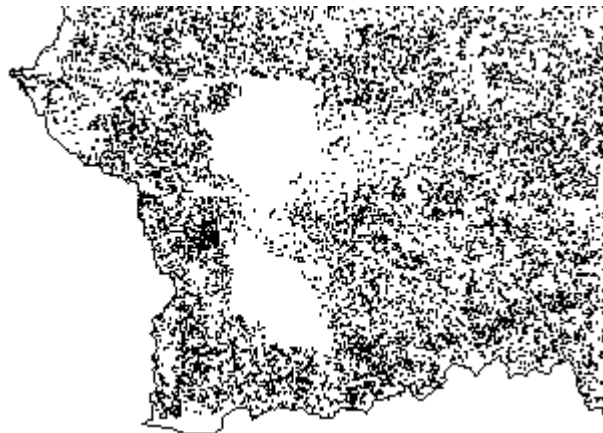
Fig. 7. Scheme of distribution of points with gravimetric measurements from the geological surveys carried out on the territory of South-western Bulgaria from 1951 to 2000 year.
