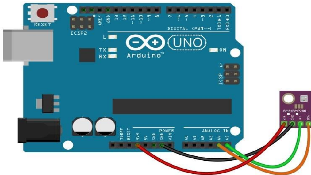
Fig. 3. Connection Arduino Uno – BME280
