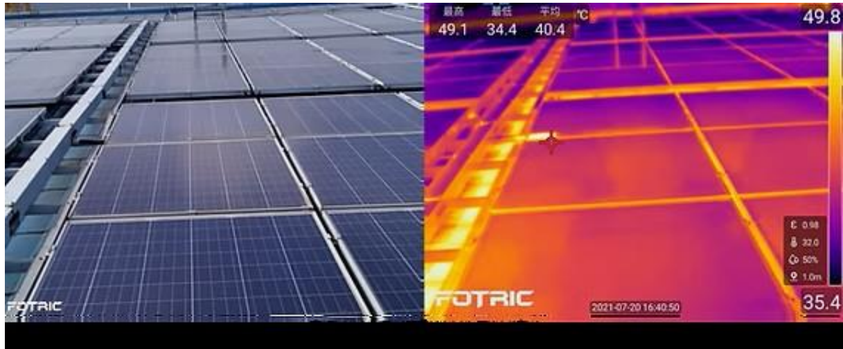
Fig. 1. Solar panel cell hotspot detection
