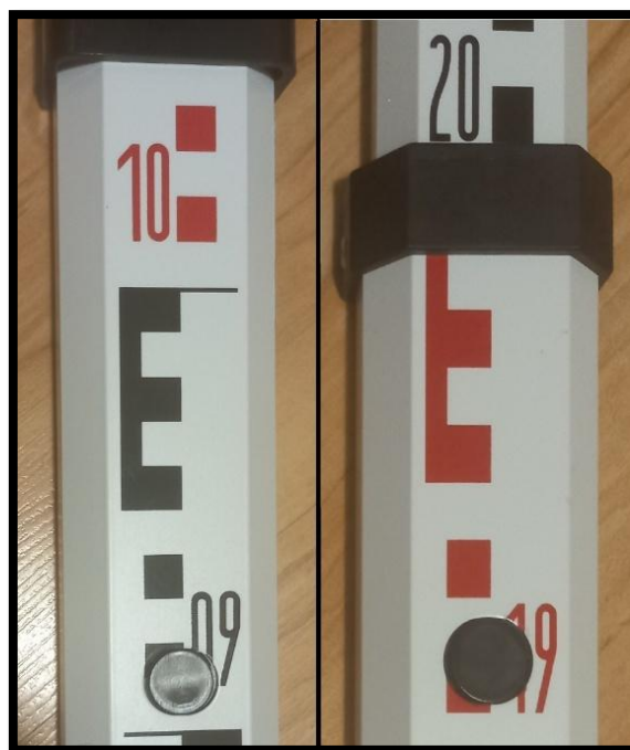
Fig. 3. Push button lock for aluminium leveling staff
