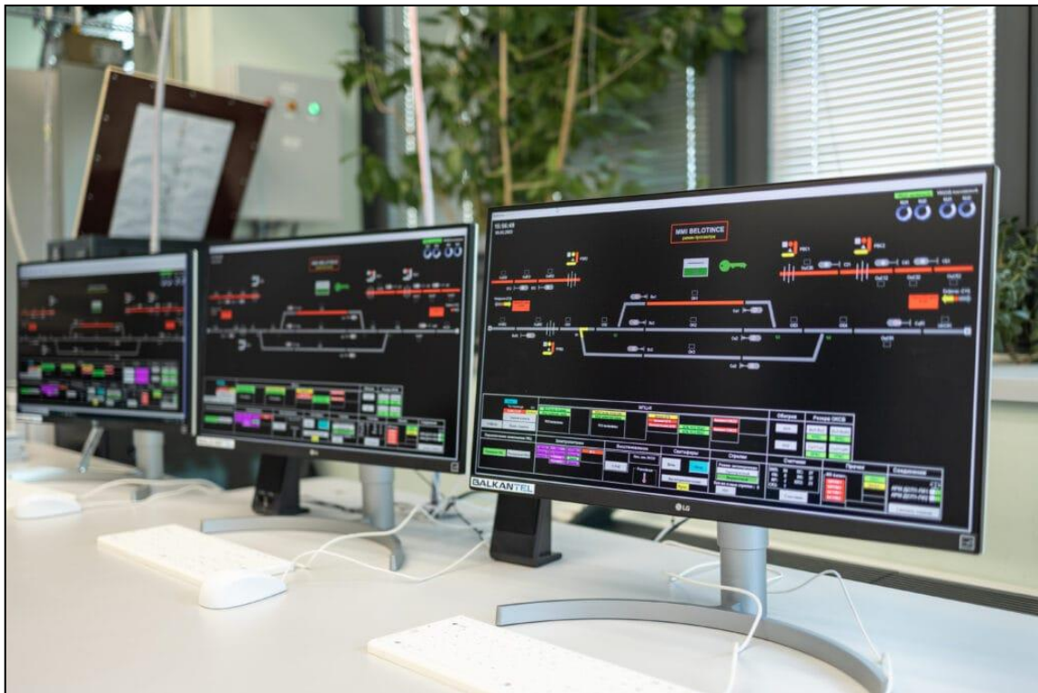
Fig. 4. Route Computer Centralization Interface [6]
